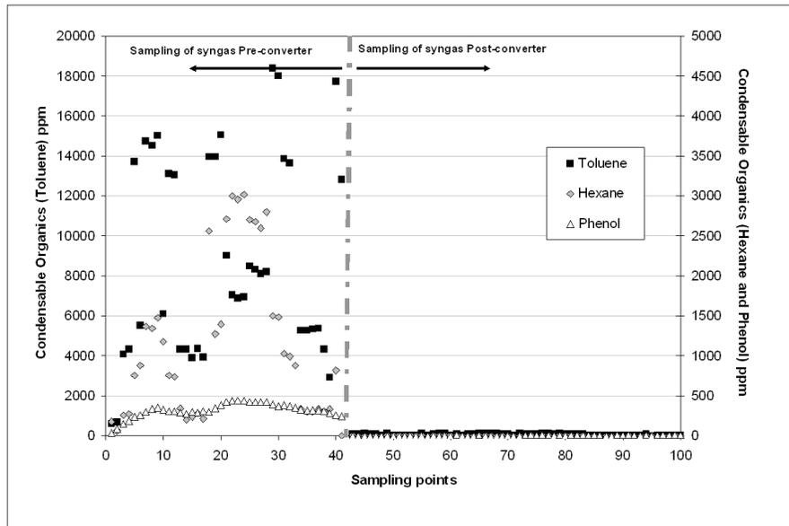
**Figure 4:** Destruction of tar-like materials within the Plasma Converter
