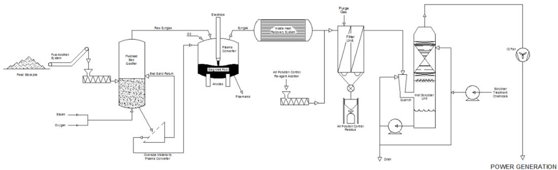
**Figure 1:** Schematic of the Gasplasma<sup>®</sup> process
