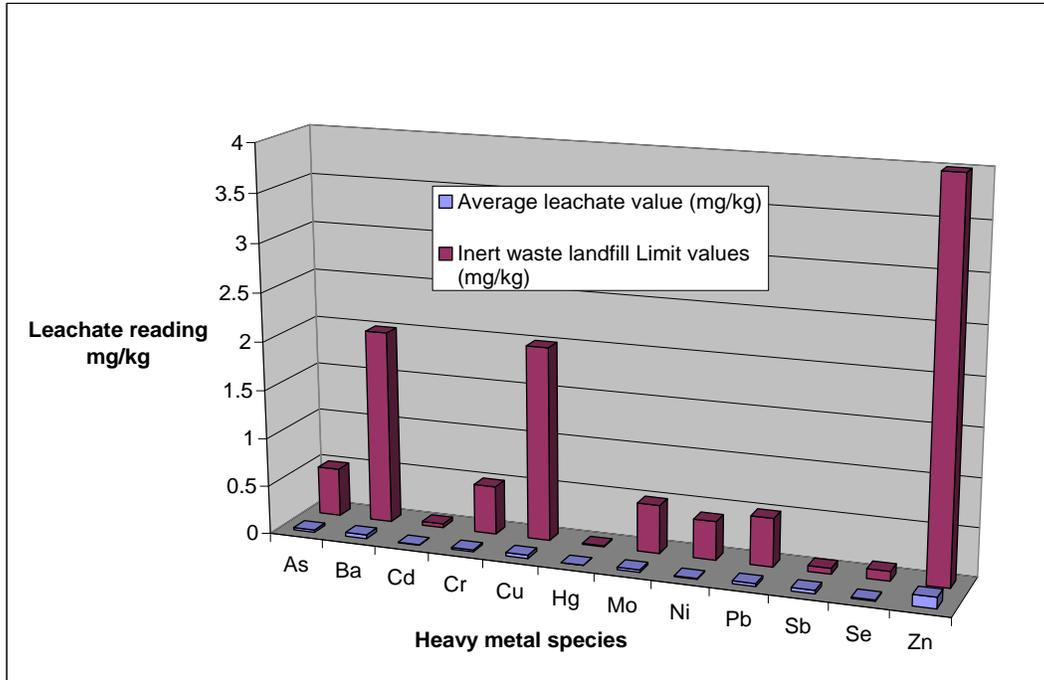
**Figure 5:** Summary of results for inert WAC limit compliance (BS EN 12457-3 Leaching tests on vitrified sample at particle size <4mm)
