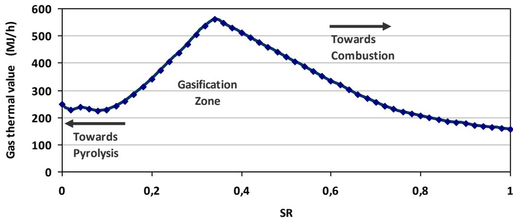
**Figure 3:** Influence of SR on gas thermal value from gasification of RDF (30 kg/h of dry MSW)
