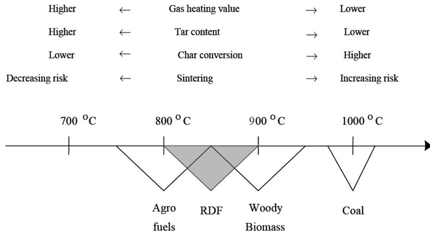
**Figure 2:** Typical gasification temperature for various feedstock and influence of temperature change on some critical factors<sup>16</sup>
